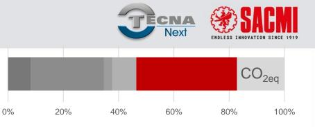
The **firing** phase shows the greatest consumption of **thermal energy** in the process and is the biggest in terms of emissions.
